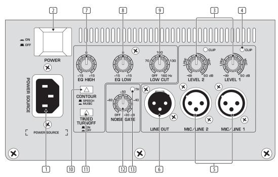
Fig. 2.1: Control elements and connections
